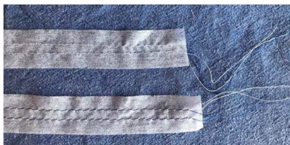
The dark blue bobbin thread is visible on the right side of the interfacing.
